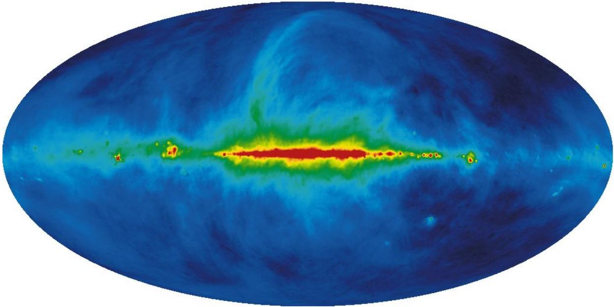
Pointing an antenna at a satellite with the center of the galaxy as a backdrop will increase the system noise by over 3dB. With a weak signal, this could become quite significant, but there is nothing to do for it other than wait for the satellite to move.
