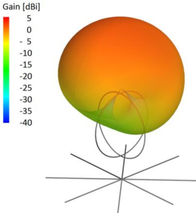
While the antenna is of a fairly low gain design (+5-6 dB), the lack of any minor lobes makes it very tolerant of noisy environments and easy to figure out the pattern as the satellite flies over.
