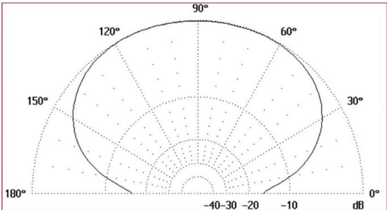
This pattern would reject much of the terrestrial noise while giving us fairly good signal in our anticipated 120 degree detection arc. What determines the pattern of the antenna is largely construction, so this becomes a process of finding the pattern which matches our use.
