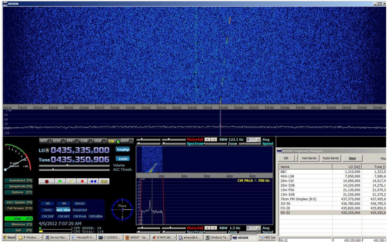
There is a satellite signal in the noise. It is the curved dashed line a little to the right of center of the waterfall display. This and other tools only show us the signal; it does not make the signal easier to receive.
