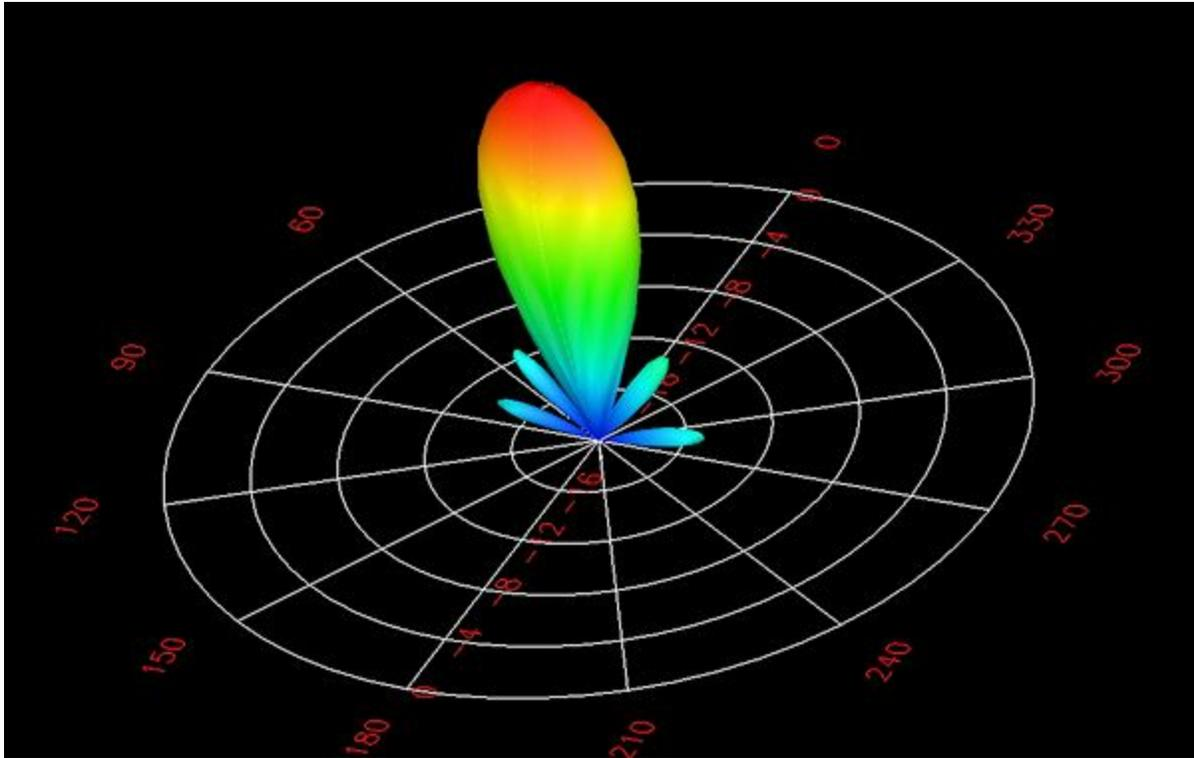
In this example, the antenna has a fairly narrow major lobe and this particular model has an efficiency of 0.88. This means that 88% of the signal the antenna has converted to electrical power is coming from the satellite, the atmosphere, and celestial objects in the major lobe pattern, while the other 12% is coming from the minor lobes.
