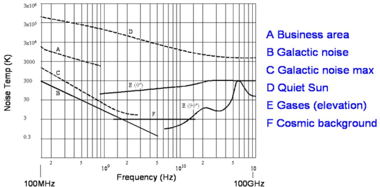
Some noise sources we do not have to worry about. For example, the earth is a fairly strong source, but if we point our antenna patterns upward and separate the antenna from the ground by a ground plane, it will not be as much of an issue. Some noise sources are best dealt with by avoiding them altogether, such as avoiding industrialized areas and not pointing the antenna at the sun.
